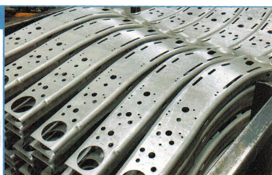
Irmco was able to show Metalsa very interesting and actionable lubricant-consumption data on two big runners, left- and right-hand siderails, for which it identified a significant difference in the amount of lubricant being applied for essentially the same part geometries. On one of the parts, adjusting the spray program and fixing the nozzle tips resulted in a 50% reduction in applied lubricant (or relative cost/part).
